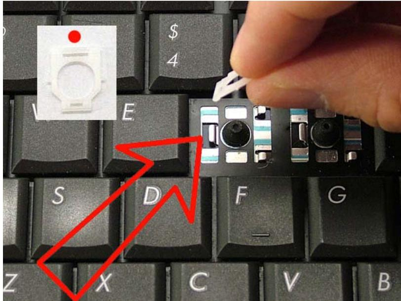
You may need to use your tool to get the hinge piece under the clip as shown in the next picture. When you are done with this step, the hinge piece will lay flat on the board, around the rubber cup, and hooked under the metal clip.
